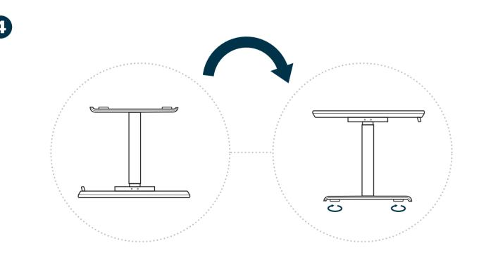
Once legs and feet are secure, two people should carefully flip the assembled desk (along the back edge to avoid damaging the control panel) to an upright position. Adjust the footpads to level the desk as needed.
