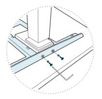
Use the smaller hex key (M6) provided to securely tighten the screws and washers (M6 - 14mm) onto each leg.
