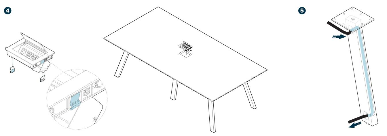
Slide the clips onto the right and left side of the power box, place it into the center of the tabletop, and press down to firmly secure them. The power unit is installed properly when it is flush with the tabletop surface.
