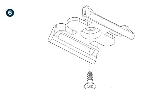
Screw the bracket into the underside of the table, in the path of the cable.
