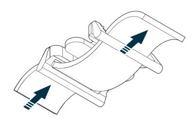
Push the velcro strap into the slots of the bracket.
